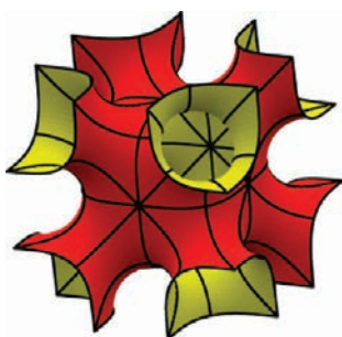
Figure 3. IW-P surface, posited as the structural element for the nanostructure of GMO-templated films after UV/O 3 treatment or acid extraction. Yellow and red signify interior volumes with 8-fold and 4-fold connectivity, respectively.
