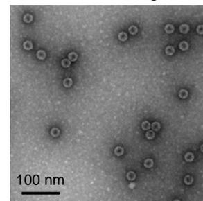
Fig. 3 TEM image of gold coated VLPs with CdSe QDs encapsulated.
