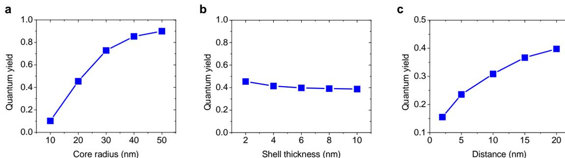
Fig. 2 (a) Quantum yield as a function of core radius when the shell thickness is fixed at 2 nm and the emitter locates at the center. (b) Quantum yield as a function of shell thickness when the core radius is fixed at 20 nm and the emitter locates at the center. (c) Quantum yield as a function of the distance from the emitter to the inner metal surface when the core radius is 20 nm and shell thickness is 6 nm.
