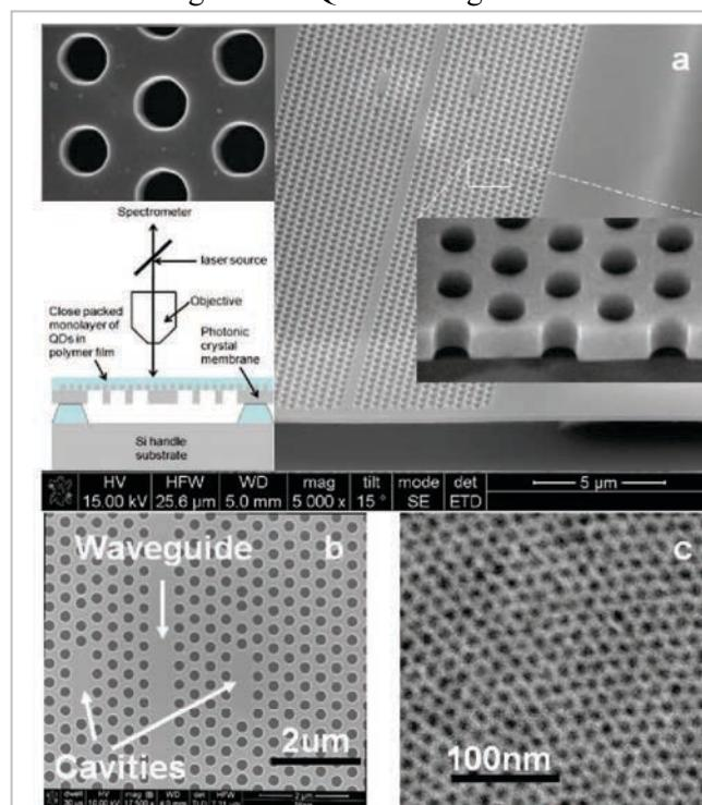
Fig. 1. (a) SEM image of photonic crystal, with upper left inset providing a detailed view of the holes (240nm diameter) and lower right inset showing the hole edges and sidewalls. The lower left inset provides a schematic diagram of the photoluminescence measurement geometry. (b) Top view of two identical L3-type photonic crystal cavities. (c) TEM image of a free-standing PbS quantum dot/P3HT polymer monolayer to be transferred to the photonic crystal surface.
