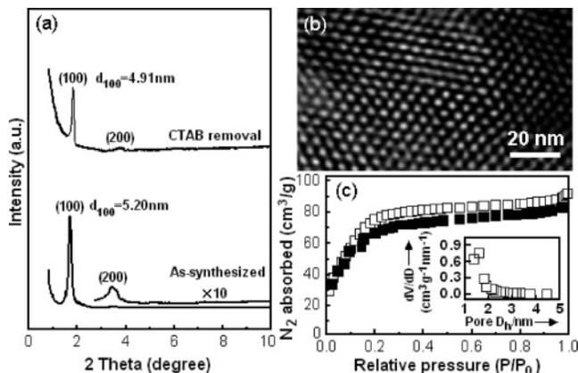
**Figure 1.** (a) XRD patterns (before and after CTAB removal), (b) TEM image, and (c) nitrogen adsorption/desorption isotherms and BJH pore diameter distribution (inset, from the desorption branch) of the PDA-PMO.
