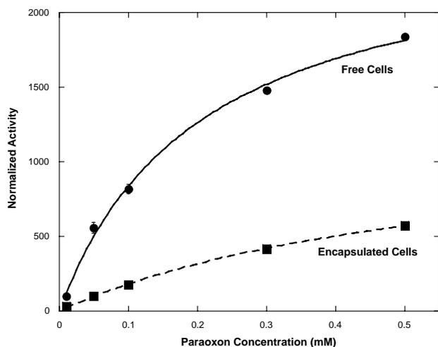
Fig. 2. Michaelis–Menten kinetics of paraoxon hydrolysis using cell-surface-expressed OPH. Comparison of free and encapsulated (sodium silicate process) recombinant *Moraxella* spp. cells. Free cells:  $K_m$ , 0.16 mM;  $V_{max}$ , 2221 AU/min OD<sub>600</sub>; encapsulated cells:  $K_m$ , 0.58 mM;  $V_{max}$ , 1232 AU/min OD<sub>600</sub>. Standard error for each data point is as shown.
