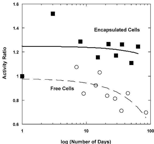
Fig. 4. Effect of long term storage on the activity of cell-surface-expressed OPH in free and encapsulated *Moraxella* spp. cells. Although encapsulation leads to lowered OPH activity as compared to free cells, encapsulated cells maintain OPH activity over a longer period as compared to free cells.
