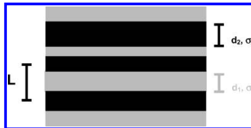
Figure 2. Illustration of a lamellar two-phase system showing the corresponding structural parameters of the SAXS analysis (see the text for the definition of the parameters).
