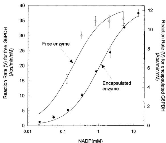
**Figure 5.** Reaction kinetics for free (○) and encapsulated (●) G6PDH at a fixed concentration of G6P and varying concentrations of  $\text{NADP}^+$ . The solid lines represent the best fit to the Michaelis–Menten equation using nonlinear least-squares regression.
