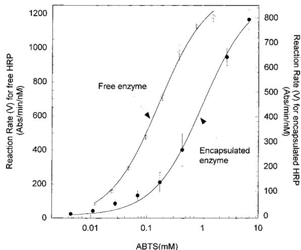
**Figure 3.** Reaction kinetics for free (○) and encapsulated (●) HRP at a fixed concentration of  $H_2O_2$  and varying concentrations of ABTS. The solid lines represent the best fit to the Michaelis–Menten equation using nonlinear least-squares regression. The curve for the encapsulated enzyme is shifted to the right, indicating an increase in the  $K_m$  of the enzyme upon encapsulation.
