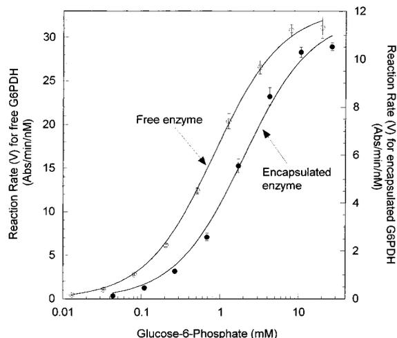
**Figure 4.** Reaction kinetics for free (○) and encapsulated (●) G6PDH at a fixed concentration of  $\text{NADP}^+$  and varying concentrations of G6P. The kinetic data were fit to the Michaelis–Menten equation using nonlinear least-squares regression.
