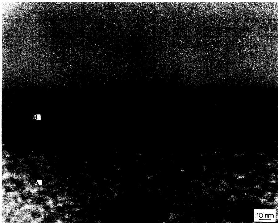
Fig. 9. Cross-sectional TEM image of a microporous silica membrane layer deposited on a U.S. Filter®  $\gamma$ - $\text{Al}_2\text{O}_3$  membrane support. Region A indicates the  $\gamma$ - $\text{Al}_2\text{O}_3$  support layer (pore size = 4.0 nm). Region B is the deposited  $\text{SiO}_2$  layer.
