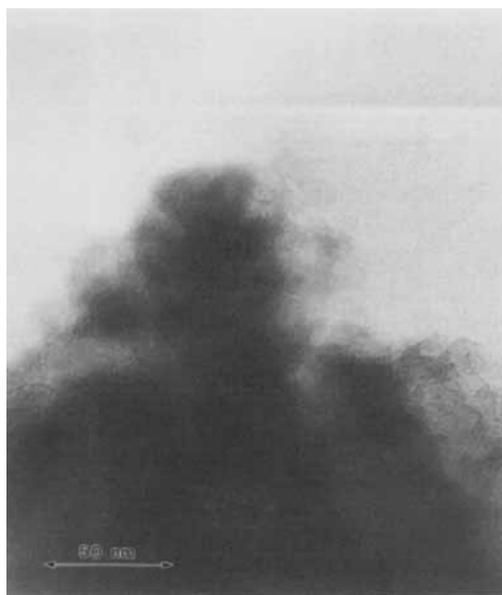
Fig. 5. HRTEM micrograph of 68 wt%  $\text{Al}_2\text{O}_3$  xerogel.
