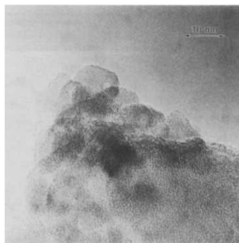
Fig. 7. Lattice fringes indicate the occasional presence of crystalline particles with dimensions of 4 to 10 nm in the 47 wt% alumina xerogel, as evident in this high-resolution electron micrograph.
