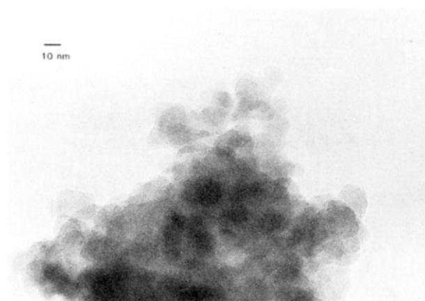
**Figure 4.** HRTEM micrograph of STO-250-2 silica xerogel.
